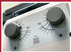
Collimator LED light that can be activated remotely or by pedal
